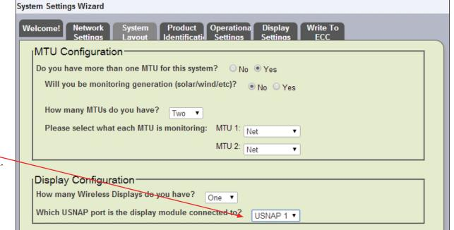
Either USNAP 1 or USNAP 2 port may be selected for use with Wireless Display. See appendix B for USNAP installation.
